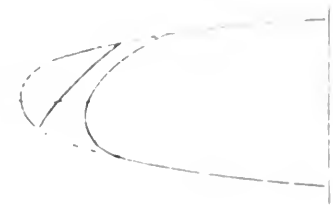
LEADING EDGE NO. 5 SAME AS CONTOUR NO. 1 SLOT ADDED REF. DWG. W.T. 179-96 5 OF 7
